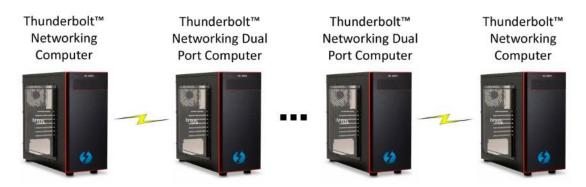
In this mode, multiple computers supporting Thunderbolt<sup>™</sup> Networking communicate through multiple Peer-to-Peer connections using Thunderbolt<sup>™</sup> 2 Dual Port hosts. In order to allow communication between different hosts in the Thunderbolt chain, network properties should be configured. We will cover two modes of operation: Bridging Mode and Routing mode.
