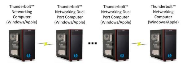
Peer-to-Peer communication is supported on OS X Mavericks version 10.9.2 and beyond, which enables Ethernet network communication over Thunderbolt with any other Apple or Windows computer that deploys a Thunderbolt 2 port. If connecting to a Windows computer, Thunderbolt Software package 2.5 or above must be installed to use Thunderbolt Networking.
